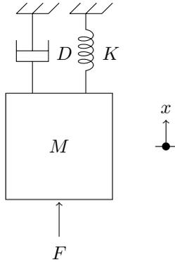
Figure 1: mechanical model of loudspeaker
