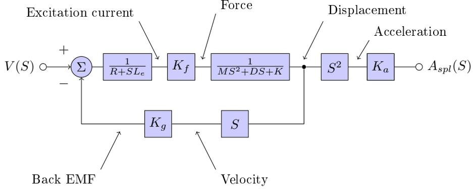
Figure 3: Dynamic Loudspeaker Block Diagram
