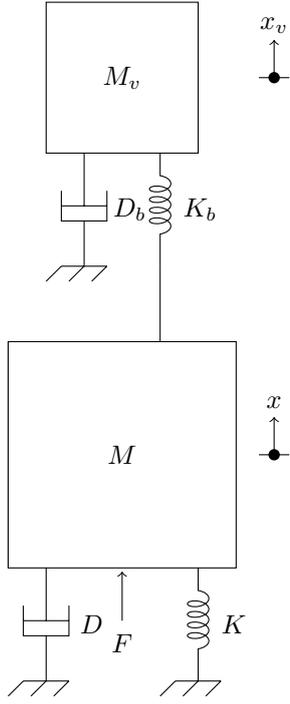
Figure 7: Mechanical Model of a Driver in a Vented Box
