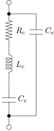
Figure 6: Impedance Equaliser Network  $Z_c$
