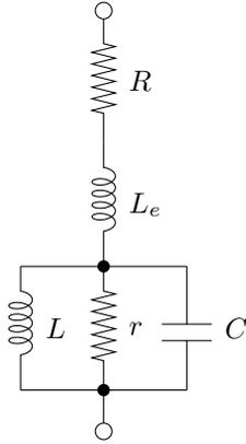
Figure 4: Impedance Presented by a Loudspeaker Mounted in an Infinite Baffle
